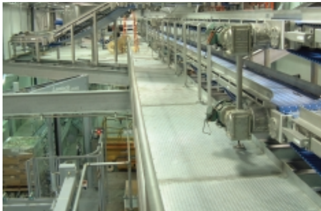
After exiting a 400' tunnel, cases are scanned and diverted to one of two accumulation lanes, which are supported by a mezzanine. Cases then merge into a single conveyor for transport to Westfalia's layer forming Palletizer.
